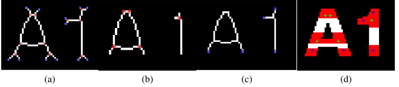
**Figure 1.** (a) Noisy thinned image with JPs and EPs detected (b)  $GI_{JP}$  times spurred image with JPs detection (c) EP detection in  $GI_{EP}$  times spurred skeletal image (d) JP and EP detection in original image with ground truth marked as red.
