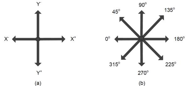
Figure 1. (a) X and Y space and reference line segments in 4-directional space (b) Reference line segments in 8-directional space.
