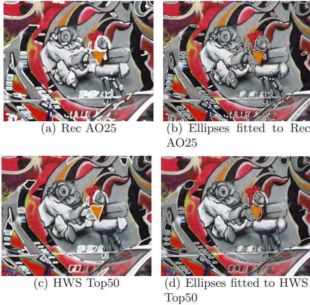
Fig. 2. (a) Outlines (in white) of the reconstruction-based morphological distinguished regions after an area opening of size 25 pixels. (c) Outlines of the 50 regions having the highest survival values. (b), (d) Ellipses fitted to the regions.
